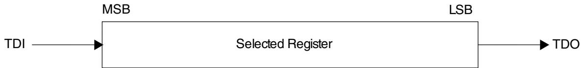
Figure 48-3. Shifting data through a register
