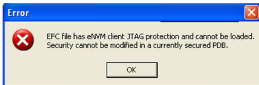
Figure 58 · EFC File with JTAG Protection Cannot be Imported into a Secured PDB Error Message
