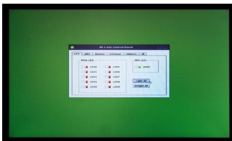
Figure 7-4 Screenshot of DE1-SoC Control Panel
